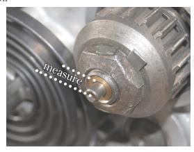
8 Refit the clutch pushrod from the timing case side (Right hand side of machine) make sure the pushrod is seated against the clutch mechanism and measure the distance the rod protrudes (pic). The rod needs to protrude from the shaft the same distance as measured in section 6 (above)
