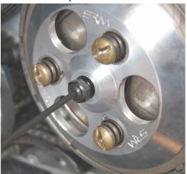
Using the marks placed on the clutch operating plunger and the clutch pushrod, line them up as shown.
