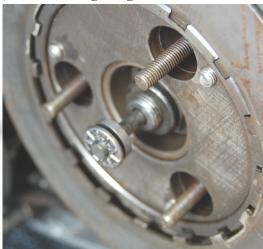
Refit the clutch operating plunger in the pushrod hole, slot end outermost and with the clutch operating lever engaged in the plunger slot. The operating lever is in it's correct, relaxed position when it's inner edge makes an approx line with the casing gasket face, as shown. With the lever and plunger making snug contact, mark the plunger in this position
